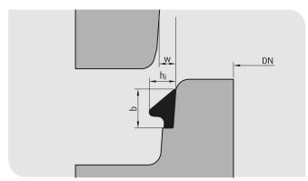
The M.O.L. concrete pipe seal system MSD is designed for concrete shafts and guarantees a reliable connection in compliance with DIN EN 1917 and DIN V 4034-1. The MSD seal also fulfils the requirements of DIN EN 681-1.
